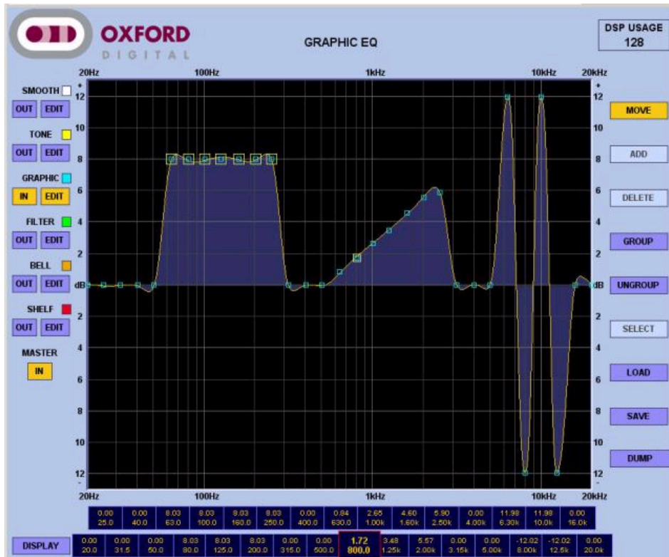
Fig. 2 Example of response of the New Graphic EQ (Yellow line shows actual response)
