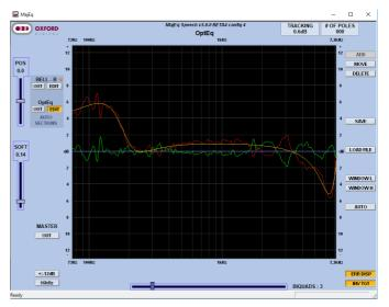
Red line: target curve required to correct the response; Yellow line: Correcting response using 3 bi-quads; Green line: Error from a flat response
