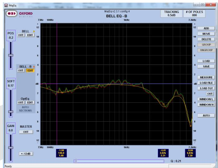
Red line: target curve required to correct the response; Yellow line: Correcting response using 3 bi-quads
