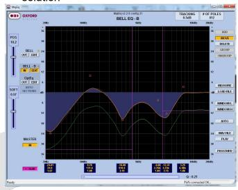
Red line: target curve required to correct the speaker; Yellow line: Correcting response using 6 bi-quads
