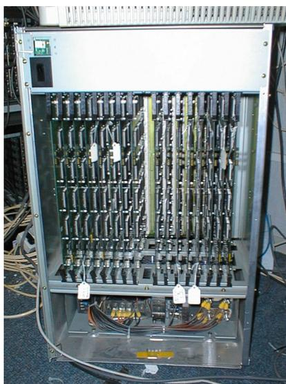
**Figure 2 Sony OXF-R3 Processing Rack**
